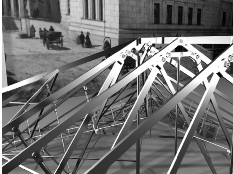
Fig 6. St. Petersburg, New Eremitage (1839-52), CAD visualisation of the roof structure above the south-western pavilion (© BTU Cottbus, Dep. for Construction History and Structural Preservation, 2003)
